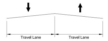
Figure 5-06: Two-Way Tangent Crown
